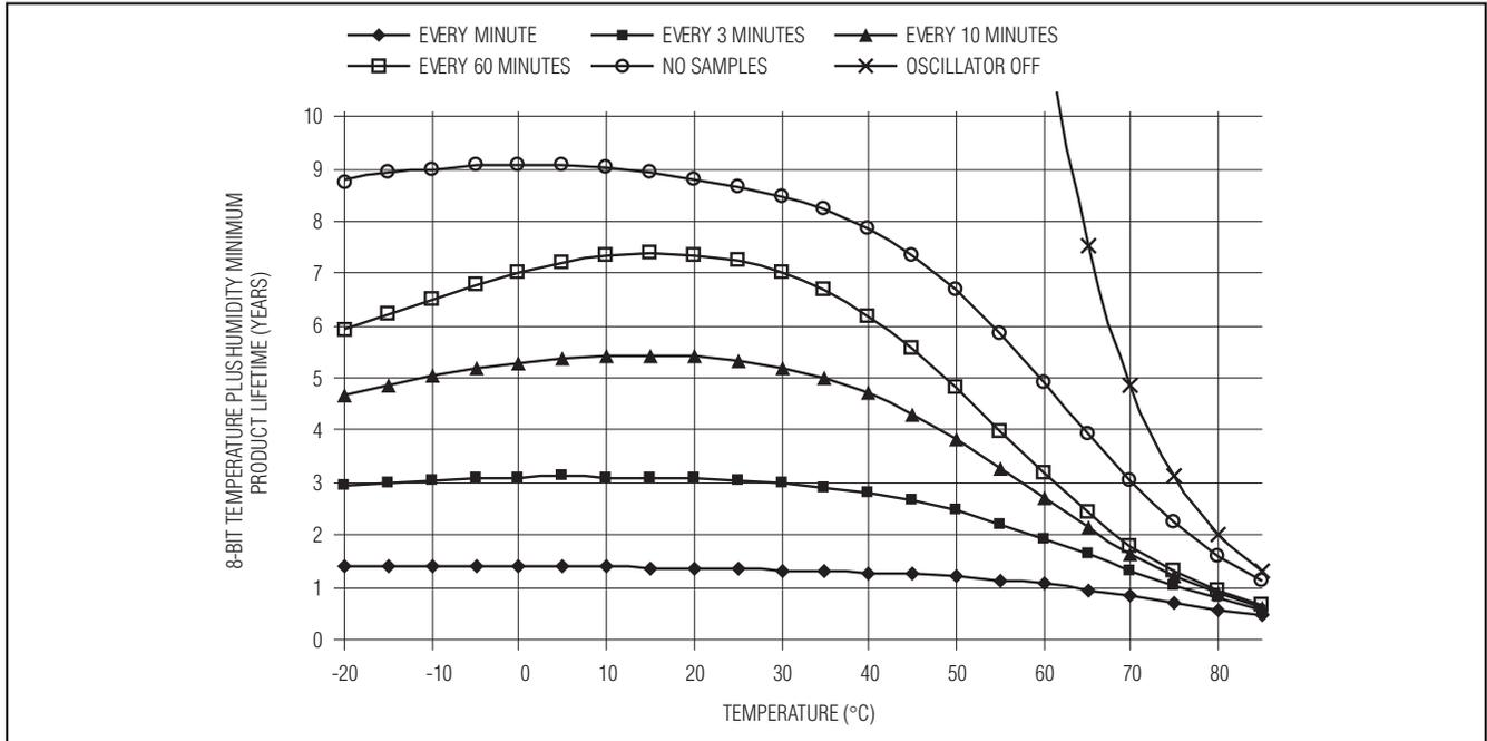
**Minimum Lifetime vs. Temperature, Fast Sampling
