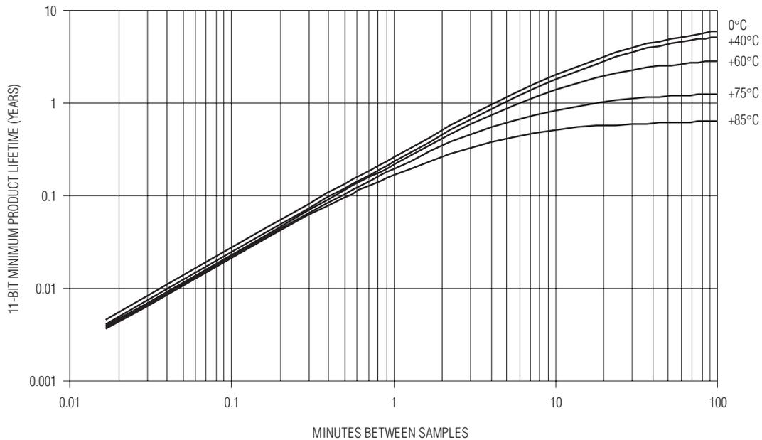
**NOTE:** WITH HUMIDITY LOGGING ACTIVATED, THE LIFETIME IS REDUCED BY A MAXIMUM OF 4%. THE INCREMENTAL ENERGY CONSUMED BY HUMIDITY LOGGING IS INDEPENDENT OF THE HUMIDITY LOGGING RESOLUTION.
