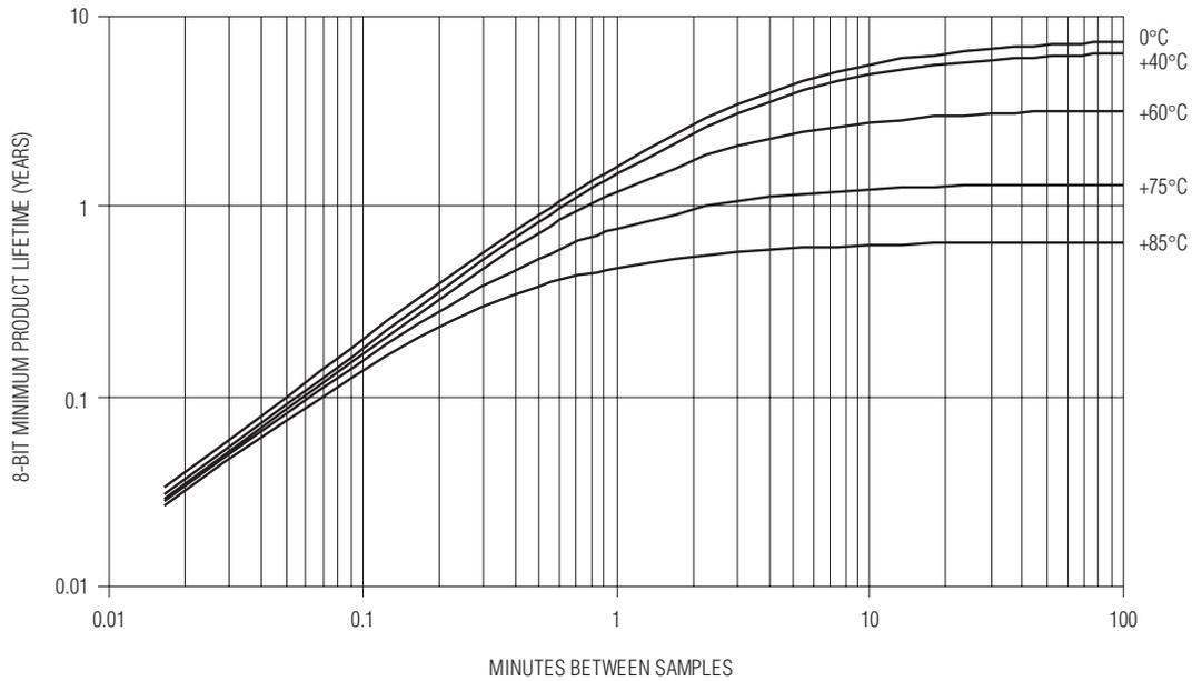
**NOTE:** WITH HUMIDITY LOGGING ACTIVATED, THE LIFETIME IS REDUCED BY LESS THAN 11% FOR THE SAMPLE RATES OF 3MIN. AND SLOWER, AND BY A MAXIMUM OF 20% FOR SAMPLE RATES OF 1MIN. AND FASTER.
