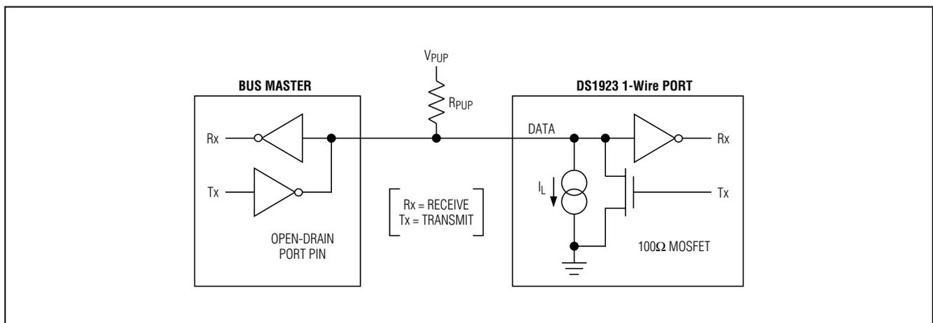
Figure 10. Hardware Configuration
