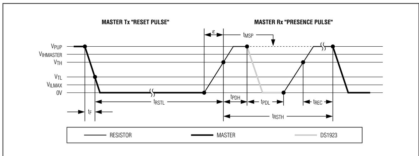
Figure 12. Initialization Procedure: Reset and Presence Pulse
